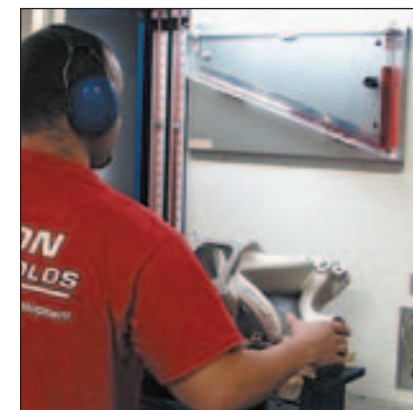
Test individual runners on V-8 intake manifolds to evaluate the balance the airflow across all eight cylinders.
