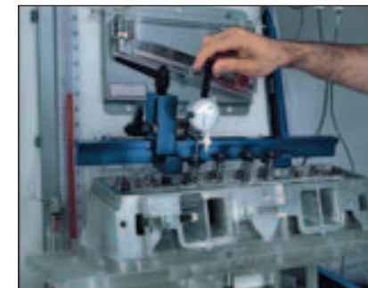
Flow test heads at different valve lifts for a more complete understanding of a port's airflow characteristics.
