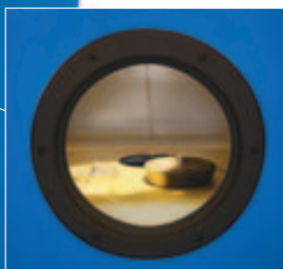
Flow-range portal A flow-range portal provides easy access to the flow range stoppers. You can change the flow range without removing your test piece from the base plate.
